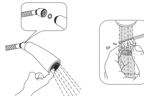
With the water running, rub the nozzles to dislodge debris.
